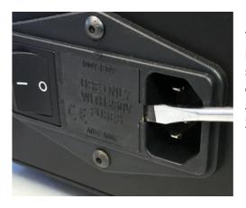
The fuse holder is in the middle of the IEC inlet. It is accessed with a small flat blade screwdriver. The holder has dual voltage designations on it and can be rotated 180° and installed to change from 100-120V to 200-240V to match your line voltage.
