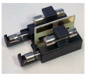
The fuse type is 5x20mm "2at" which is a 2 amp "slow blow" device. Spares are held inside the slide out compartment. Both the hot and the neutral lines are fused so make sure to check both if the unit will not power up. Fuses are safety devices and it is not unusual for one to occasionally blow and this should be the first thing to check if a unit will not power up.
